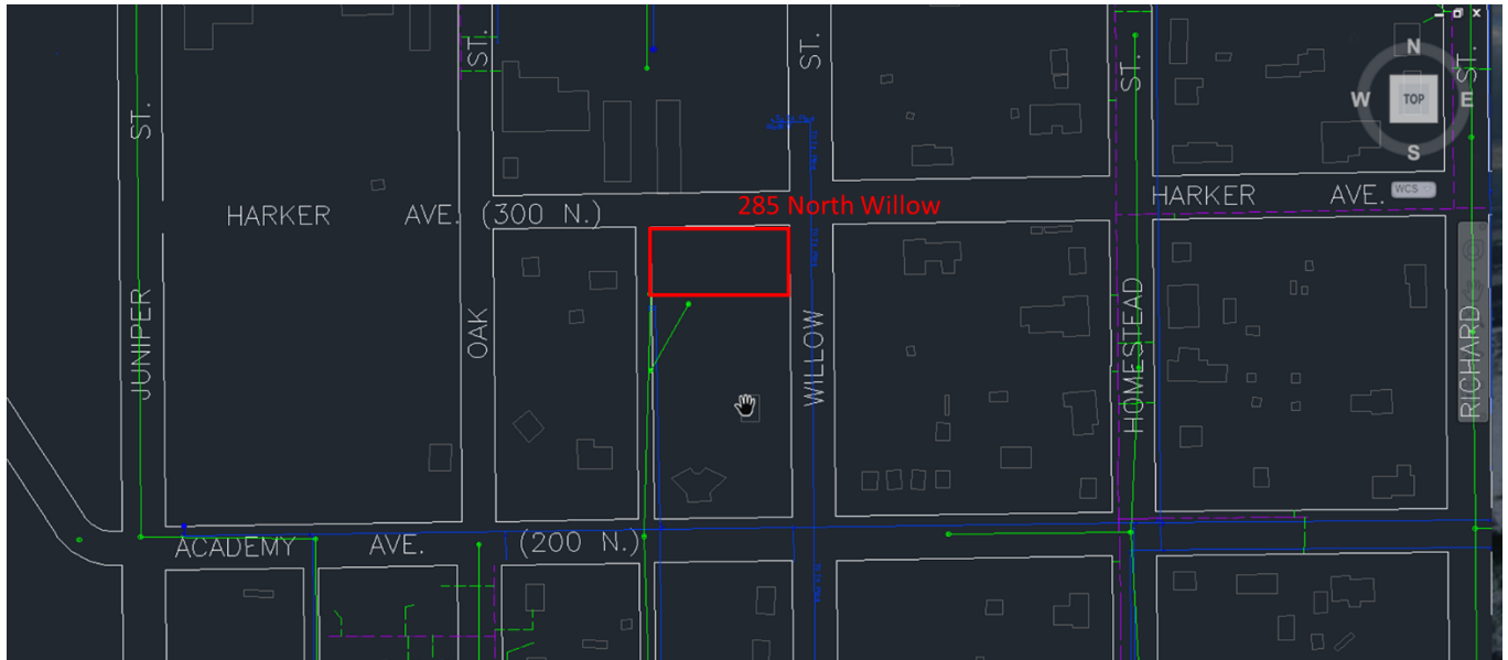
Figure 1 285 North Willow Street; Green Represents Sewer Service, Blue Represents Water Service, Purple Represents Gas Service
